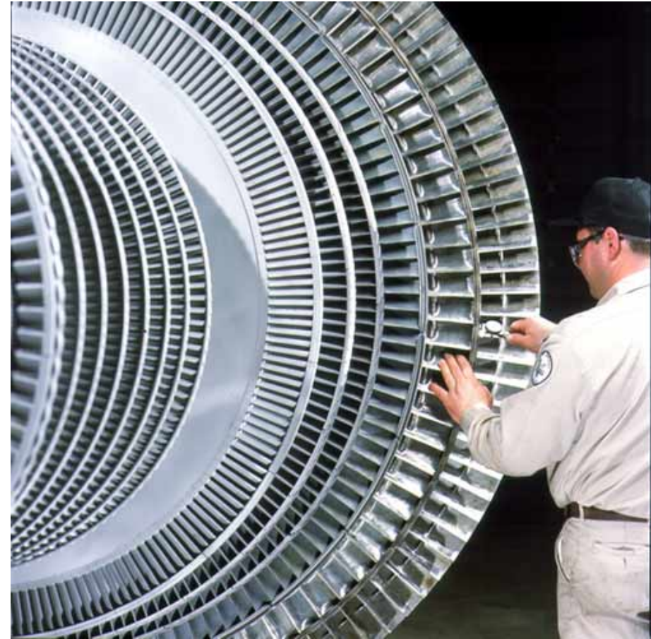
Refurbishment and Repair of a Steam Turbine – © Sulzer Metco
